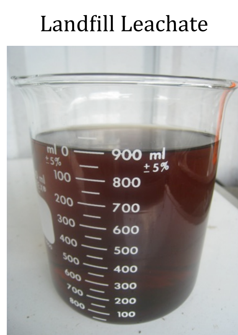
Figure 1. Landfill leachate is a dark-colored, odiferous liquid rich in ammonium, potassium, and trace metals.
